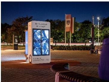
Public book exchange for local readers with renewable energy. The structure of the cabinet is powder-coated aluminum, the doors and the solar panel are covered with safety glass. The doors are closed by gas springs. The lighting of the larger cabinet is provided by solar panels and LED light, and its operation is ensured by twilight and time switches. Installation of a Wi-Fi hotspot for the adult version is optional.
