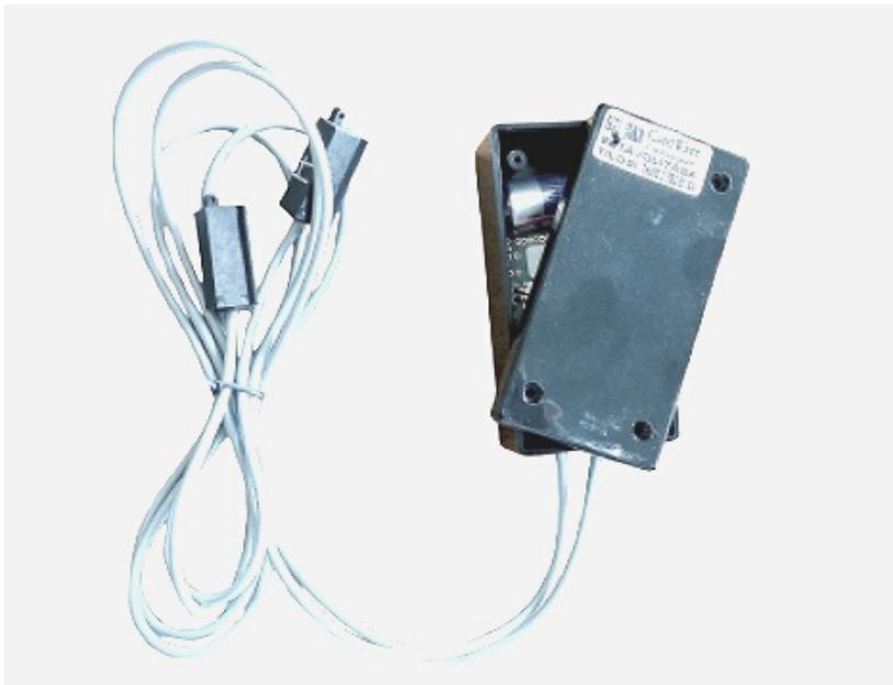
*A two input RF unit for remote meter-reading of water meters.*
