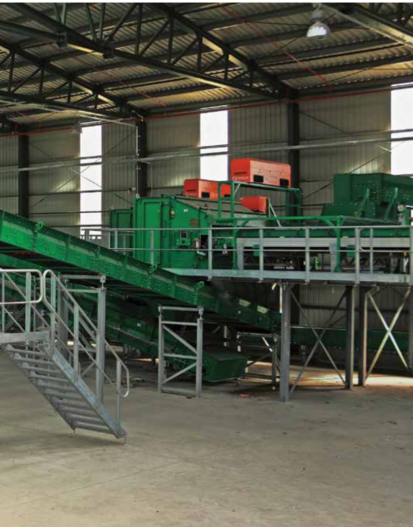
Sorting system with drum screen, NIR and Eddy current separator
