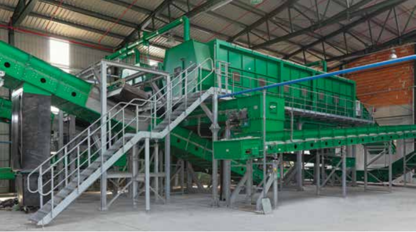
Sorting system with drum screen, NIR and Eddy current separator
